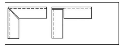
Methods of the ends of two equal angle iron bars that have to be welded at 90° to each other.
