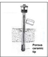
2.2.1 During the measurement of soil water tension, the water seeps through the ceramic tip of the device to measure soil water tension. Describe the difference in the rate of water seepage from the ceramic tip into the soil in a dry and in a wet soil.
