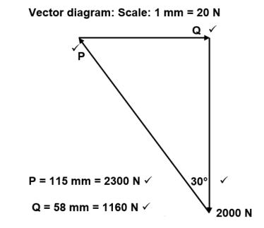
Horizontal and vertical components of a force acting at an angle.
