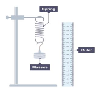
Different masses are suspended, and the corresponding elongations are obtained.
