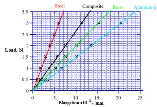
Which one of the following materials has the greatest modulus of elasticity?
