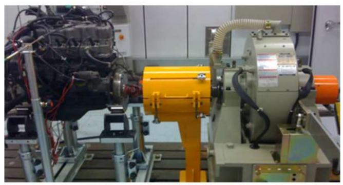
Eddy current dynamometers use a magnetic field to provide counter restraining torque that increases with shaft speed.
